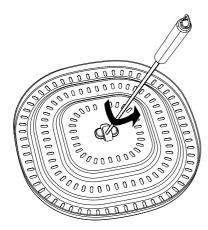
Hold the fire hook vertically to the ground, ensuring that the head of the fire hook perfectly fits into the positioning groove of the fire ring. This will allow you to successfully remove the fire ring.
