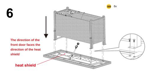
Do not lock all the screws at first, and lock them after all the mounting holes are aligned.
