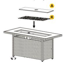
Use the four adjustable leveling feet to adjust the tabletop flatness. Clockwise for lower level, counterclockwise for higher level.
